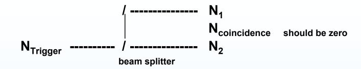
When the beam splitter sends non dividable photons unambiguously into either path 1 or path 2, N<sub>coincidence</sub> should be zero.
