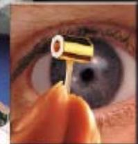
**4** Slices of giant crystals convert the infrared lasers to ultraviolet light before the beams enter the target chamber.
