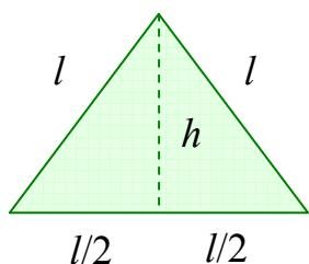
$$(11) \quad h^2 = l^2 - \left(\frac{l}{2}\right)^2 = \frac{3l^2}{4} \quad \text{entonces} \quad h = \frac{l}{2}\sqrt{3} \quad \therefore \quad h = 6\sqrt{3} \text{ cm}$$
