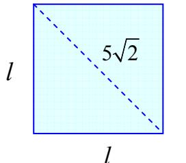
$$d^2 = 2l^2 \text{ entonces } l = \frac{\sqrt{2}d}{2} \therefore l = \frac{\sqrt{2}(5\sqrt{2})}{2} = 5 \text{ m.}$$
