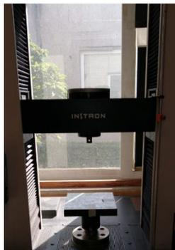
Figura 5. Máquina Universal INSTRON-40502
